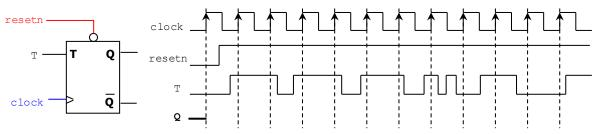
• Complete the timing diagram of the circuits shown below: (7 pts)
