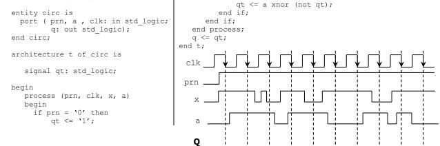
The following circuit is a single-input compressor circuit (SIC), a component in Built-in Self-Test systems. Complete the timing diagram of the following circuit:  $Q = Q_3 Q_2 Q_1 Q_0$  (10 pts)
