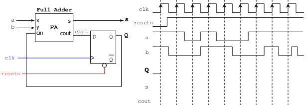
Complete the timing diagram of the circuit shown below: (7 pts)
